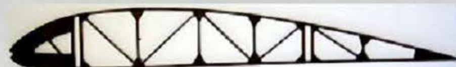
Wing rib for the Triad. While the fuselage was built of steel tubing, the wing was wood. Rib had a generous 84-in chord and was 11-in thick. Vertical slots are where the wing spars passed through. Rib was labor intensive, requiring lots of gluing and pinning with small brads at the gusset joints.
