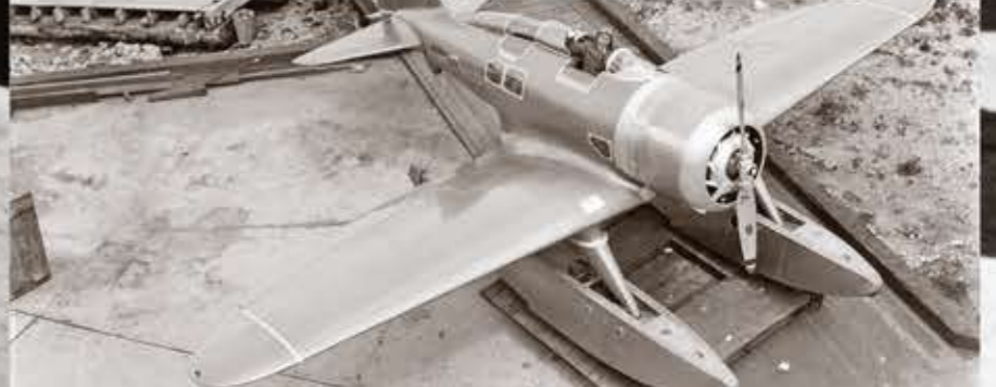
Seversky waves from the cockpit of the SEV-3. This view shows how the struts could move within the floats, thus changing the angle of the aircraft.
