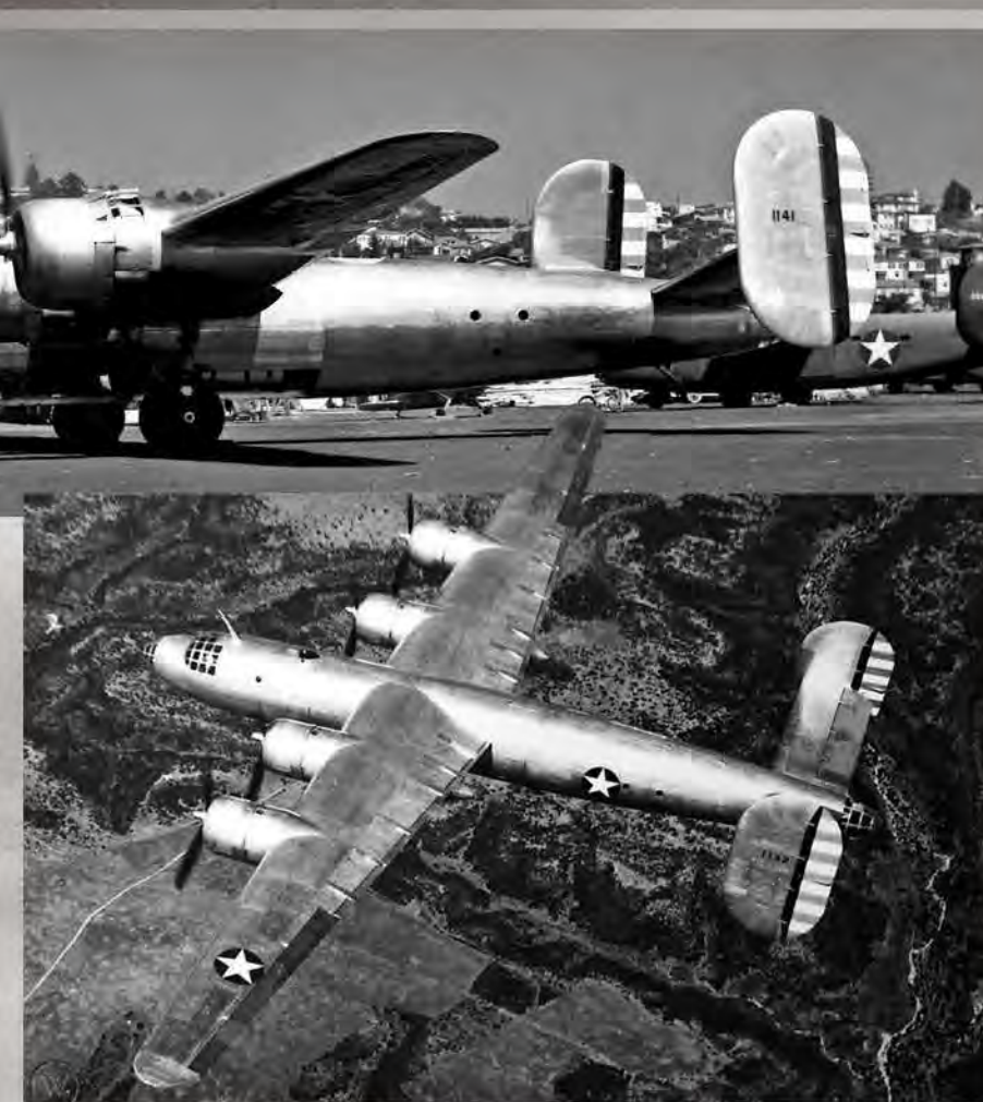
This view of the prototype illustrates the Davis high-aspect ratio wing to advantage. (Convair)
