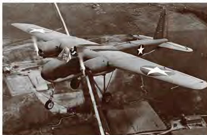
Lieutenant Corley displays the TDN-1 in flight near NAS Traverse City. The design was supposed to be as simple as possible while the wood and other non-strategic materials used in construction would not hamper the production of combat aircraft. This view shows the broad wing to advantage.
