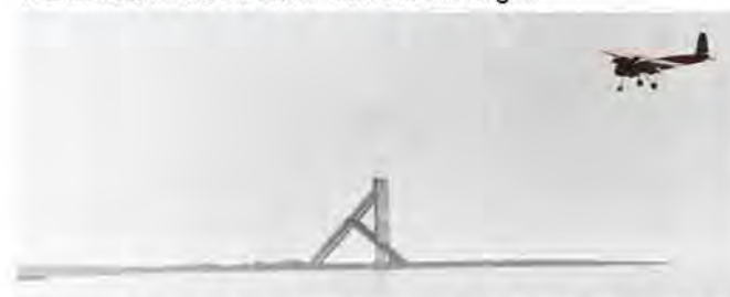
Other tests saw the bomb-laden TDNs flown directly into the target to test the effectiveness of such an attack.
