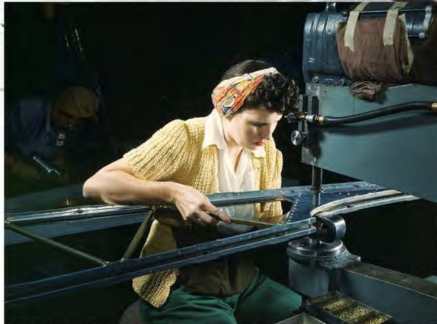
At the Douglas factory, a female employee carefully aligns Fortress wing ribs during fabrication. The wing of the Fort was exceedingly strong but was vulnerable to fires started in the Wright Cyclone radials and associated turbosuperchargers. If a fire began in the wing — due either to a component failure or combat damage — the onboard fire extinguishers were often inadequate to extinguish the blaze, leaving the crew no choice but to escape by parachute if there was time.
