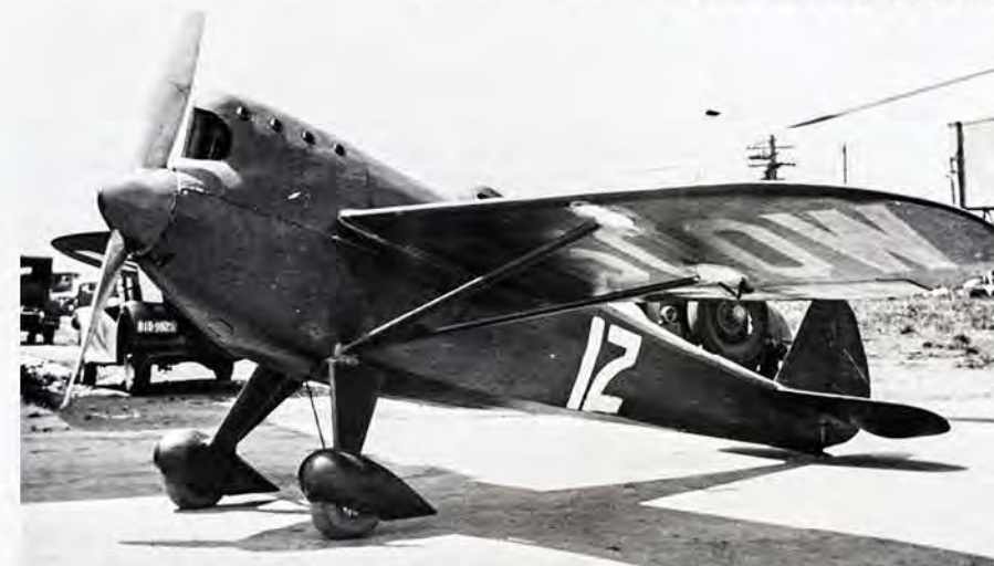
For the 1933 season, the Mono-Special became the SK-1 or Folkerts Special with a cutdown wing, modified gear, small tires, and equally small streamlined wheel coverings. Note the crudely applied race number.
