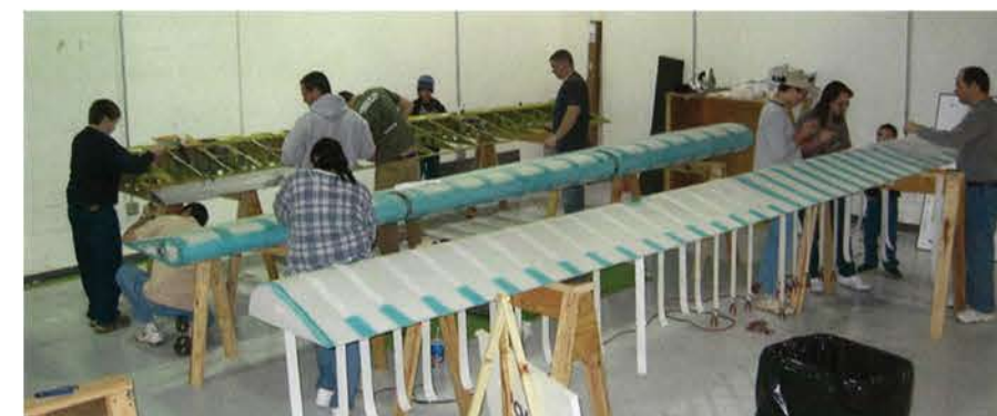
Volunteers from LMI Corporation mounting fabric on the ailerons and elevators under the supervision of volunteer David Pinegar.
