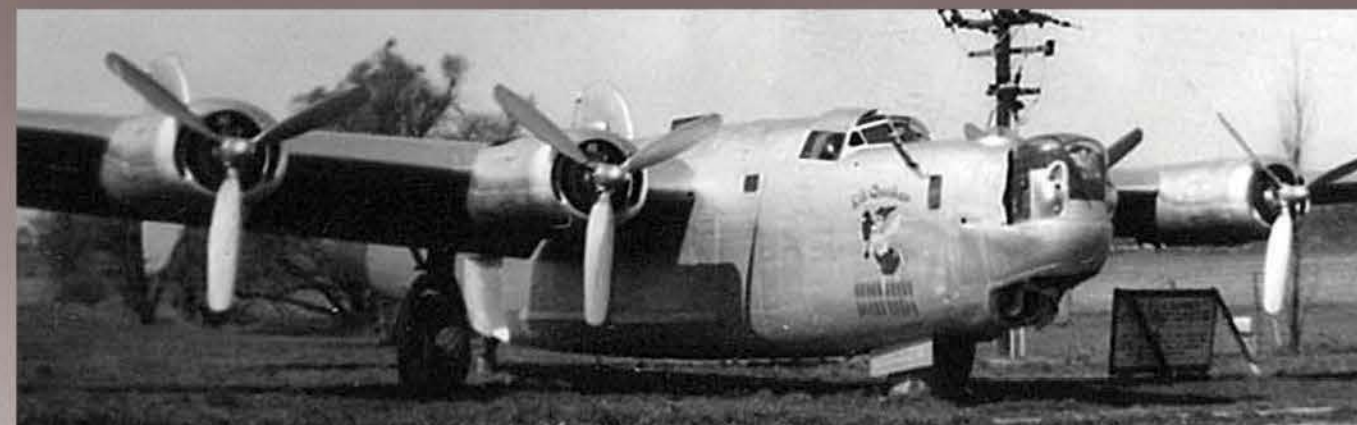
Reader Tom Kirk of Meadville, Pennsylvania, identified number 27 as Ford-built RB-24E 42-7217, and that it wore the name Lil Quaker when serving as a memorial. Notice the fuselage cut-out under the waist window.
