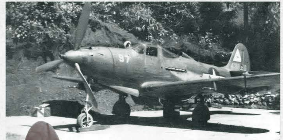
During WWII, Airacobras fought long and hard in remote and dangerous combat zones. P-39Q 44-3866 was assigned to the 28th Fighter Squadron. As long as P-39 pilots did not try to dogfight with Japanese opponents or take the fight to over 12,000 feet, they enjoyed a number of advantages such as self-sealing fuel tanks, armor protection, heavy armament and an Allison V-12 that offered good low-altitude performance.
