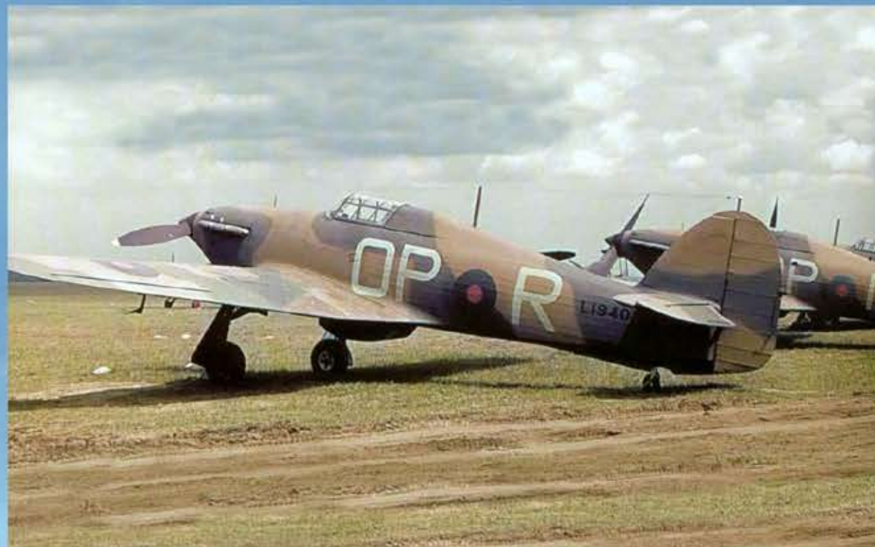
Rare early color image of a Hawker Hurricane Mk. I. Serial L1936 was out of the first production batch of 50 of the RAF's first monoplane fighter. Fitted with a fixed-pitch wooden propeller, the Hurricane carries the OP codes of No. 3 Squadron. The camouflage was for 1938's Munich Crisis but when the war started in September 1939, squadron codes change to QO. By the middle of 1938, the first 50 Hurricanes reached squadrons but the type was being delivered faster than the RAF could absorb them into squadron use. By the time of the Munich Crisis, only two of the projected twelve Hurricane squadrons were operational. By the start of the war, there were 18 operational Hurricane squadrons with three more converting.
