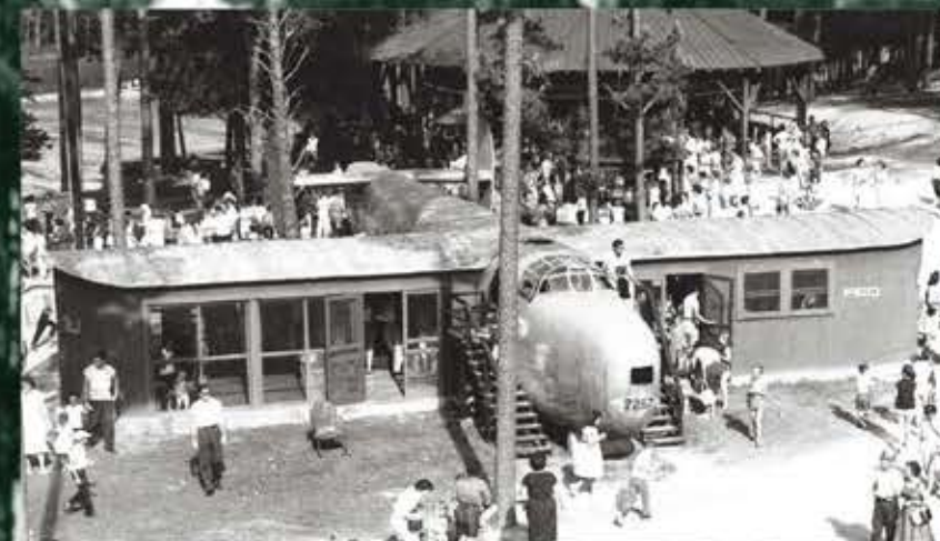
The Springs Park Liberator, C-87 42-107257, served as a hot dog stand for years at the amusement park. The fuselage was the kitchen and new-build wings served as the roofs over screened-in eating and display areas. (Springs Close Family Archives)
