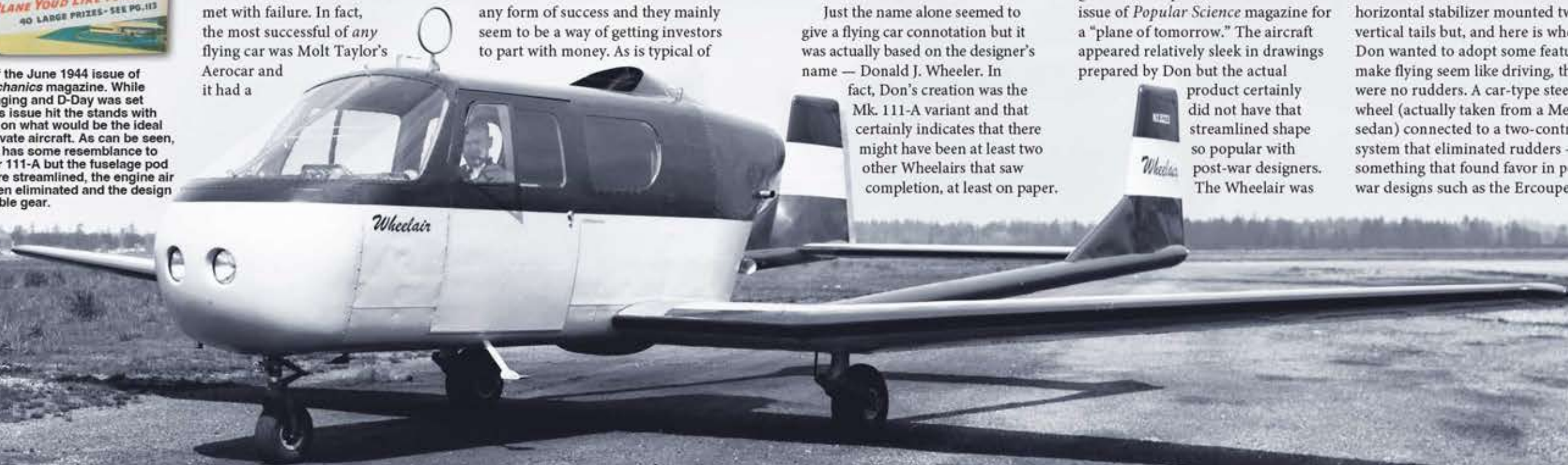
With the 190-hp Lycoming running up, the Wheelair 111-A prepares for a test flight. All the trim on the aircraft was bright red. Note the large twin landing lights in the nose — another feature with a car-like appearance.
