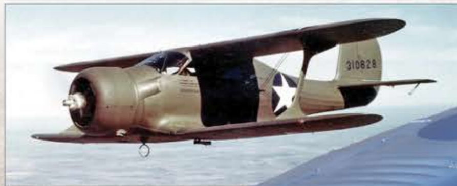
Beech UC-43 43-10828 of the USAAF. Aircraft is painted in standard USAAF Olive Drab/Neutral Gray
