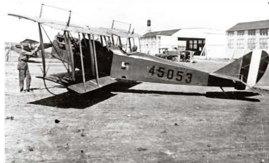
The Curtiss JN-4H was the 120th Observation Squadron's first aircraft. However, the high altitudes near Denver were too much for its limited performance.
