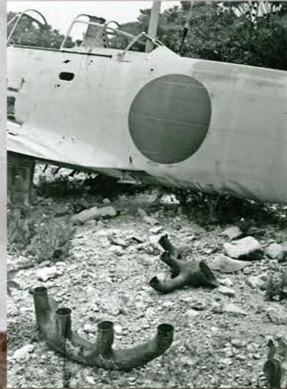
Surrounded by rusty exhaust collectors, a Marine photographer took this detailed photo of the hinomaru on a lesser damaged Zero.
