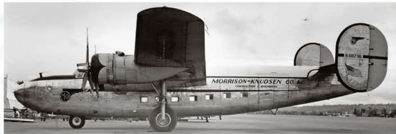
Photographed during the 1953/1956 timeframe, Liberator AL557/N68735 displays its passenger modifications. Note that the bomb bay has been modified, passenger windows added, along with a two-door cargo hatch in the fuselage. The nose has also been modified into a cargo hold and the nose cone would swing open for easy access. Note the Morrison-Knudson logo, flag, and registration on the vertical stabilizer. (Nicholas A. Veronico Collection)
