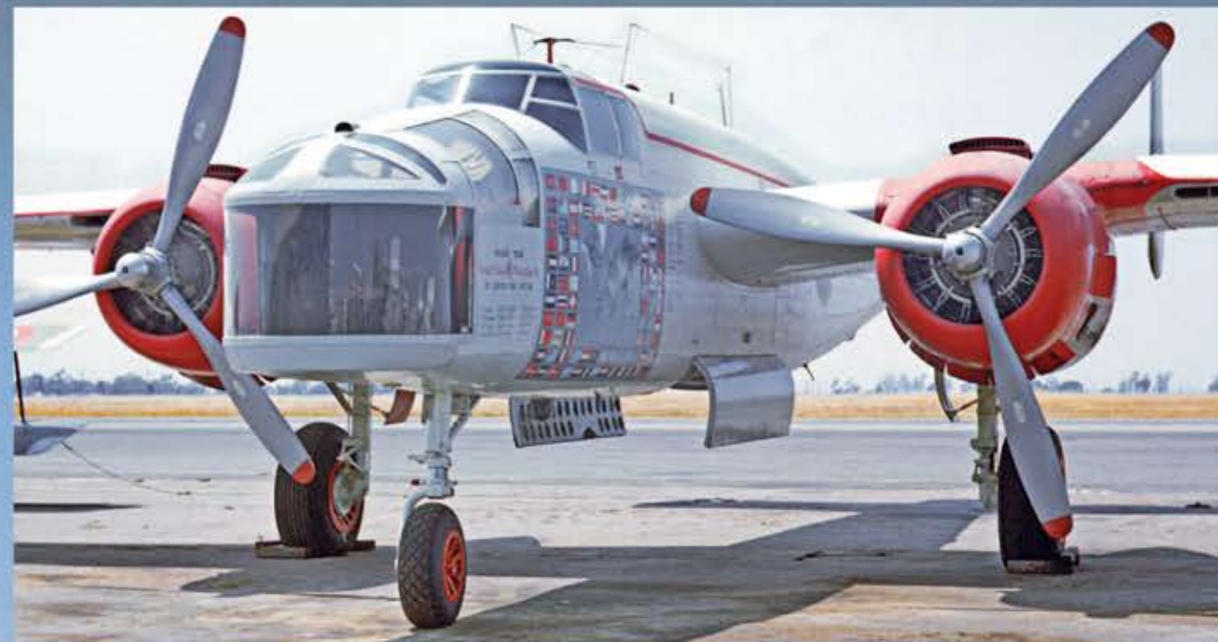
B-25H The Smasher on the Paul Mantz Air Services ramp in June 1961. Detail of the custom Cinerama nose are clearly seen with the wrap-around nose glass and the additional windows. The B-25H wore this scheme from 1956 until it was repainted by Tallmantz after the company was established in November 1961. (J.D. Davis)
