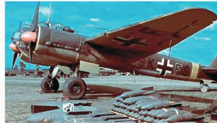
The Ju 88A was a formidable weapon that could perform numerous tasks. It was fast, had a good range, and could tote a reasonable bomb load. It had a weakness in its poor defensive armament. Unlike the Americans, the Germans never really developed an effective defensive armament for their bombers. This example, waiting to be bombed up, has been modified to carry an extra rear-facing 7.92mm weapon along with a forward-facing similar weapon.
