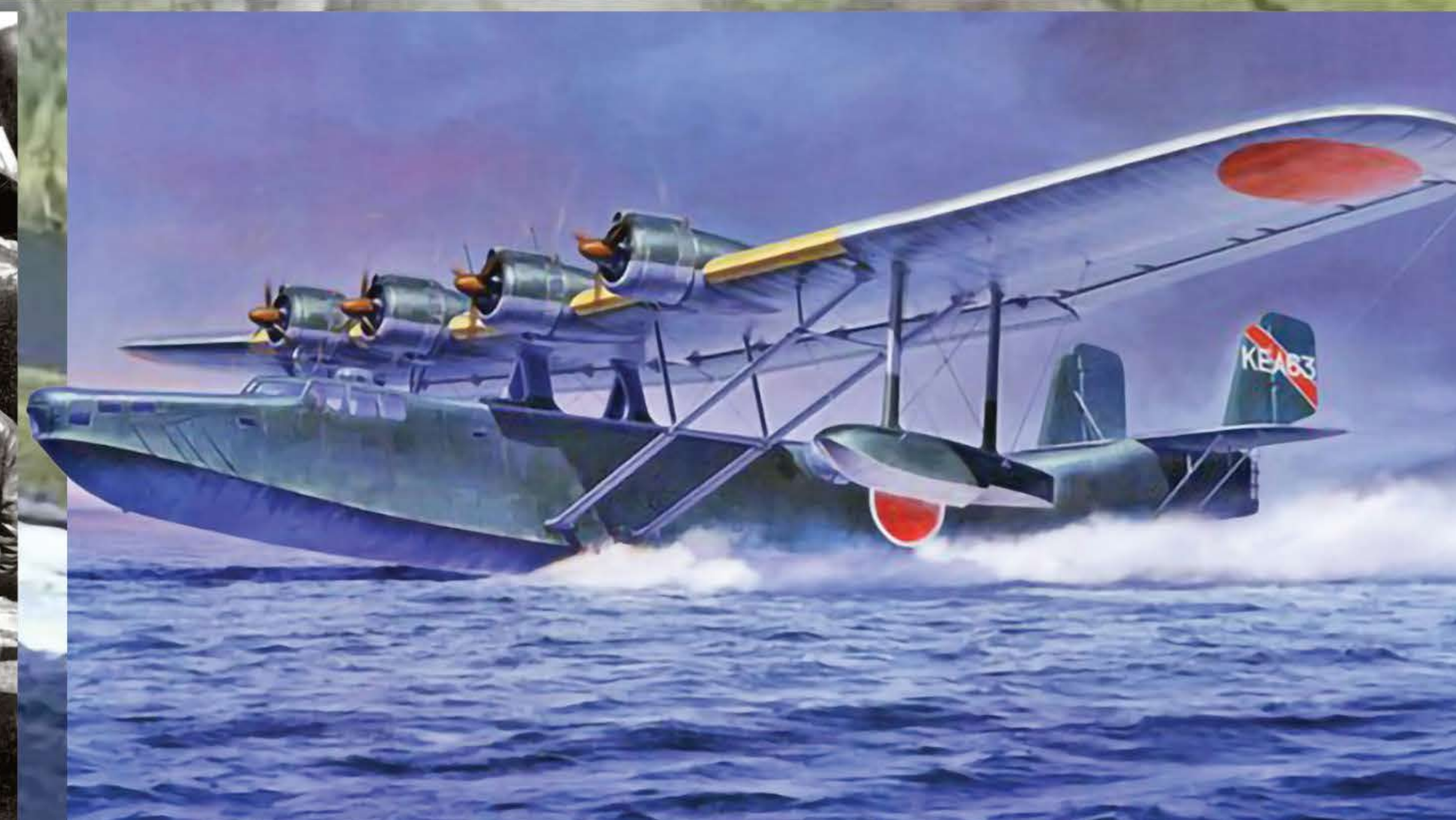
The Mavis was relatively heavily armed and carried one Type 92 .30-caliber gun in the nose, two Type 92s in the waist position, one Type 92 atop the fuselage, and one Type 99 Mk. 1 20mm cannon in the tail position.
