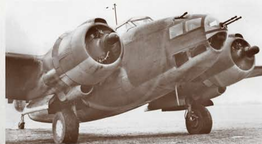
This view of a standard RAF Ventura shows the stock nose, added armament, and Pratt & Whitney R-2800-S1A4-G powerplants of 1850-hp each.
