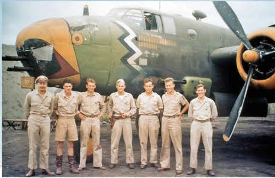
Crew of a 498th Bomb Squadron "Air Apaches" B-25D Mitchell with their attractively painted but well-weathered aircraft. As can be seen, the plane's glass nose has been painted over and four .50-caliber machine guns have been added along with the early style cheek guns that held two .50-caliber weapons each. Note the aluminum flak-damage patch on the forward nose.
