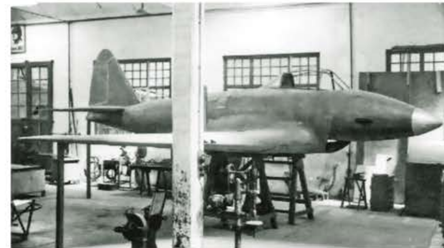
The mock-up in the Piaggio factory. Note that wing guns are installed but no weapons are mounted in the nose section.
