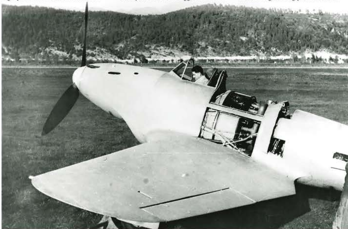
Preparing for engine start. Note the overall clean metal work and this view shows how the engine was mounted directly behind the pilot. Also note that only two guns are installed in the nose.
