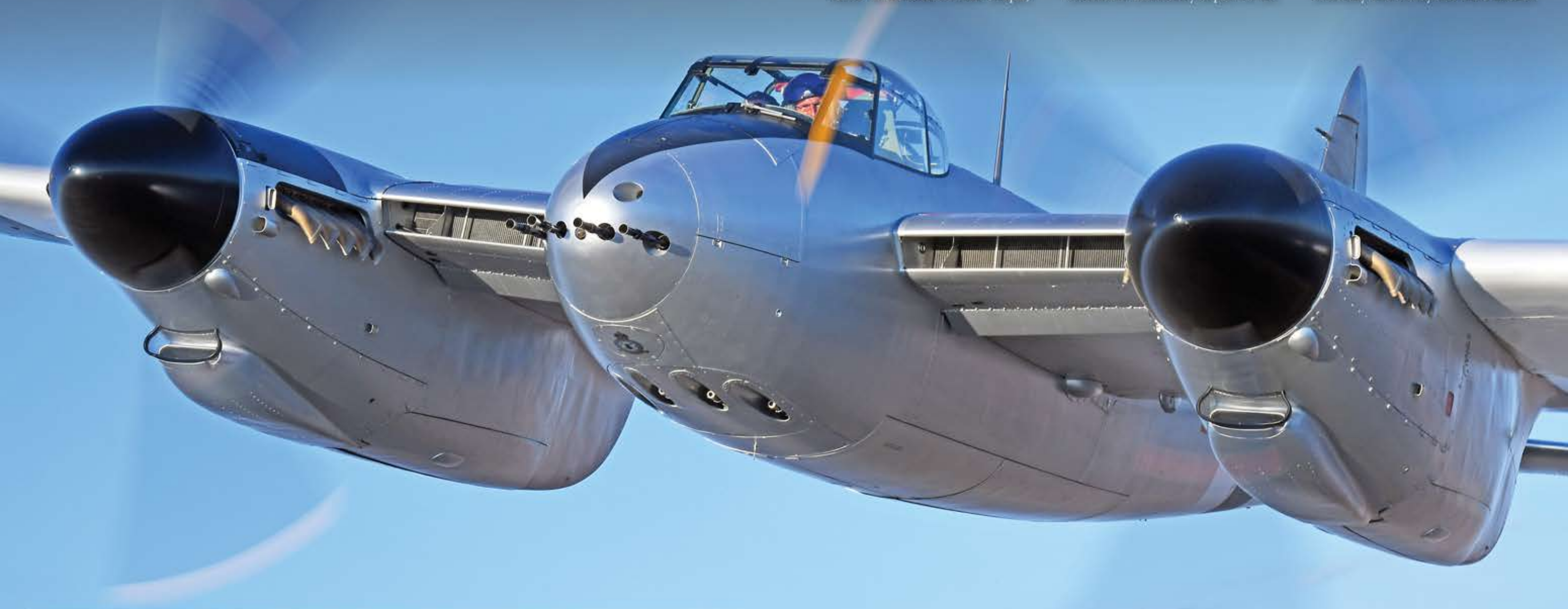
Steve Hinton brings NZ2308 in tight on Bradon Kunicki's SNJ flown by Pat Nightingale. This view shows the concentrated firepower of the four .303-caliber machine guns and four 20mm cannon.
