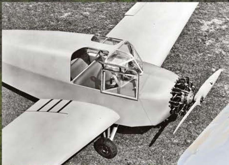
High-angle shot of what is probably the first Si 202. Note the extremely smooth finish to the aircraft and the French Salmson radial engine.
