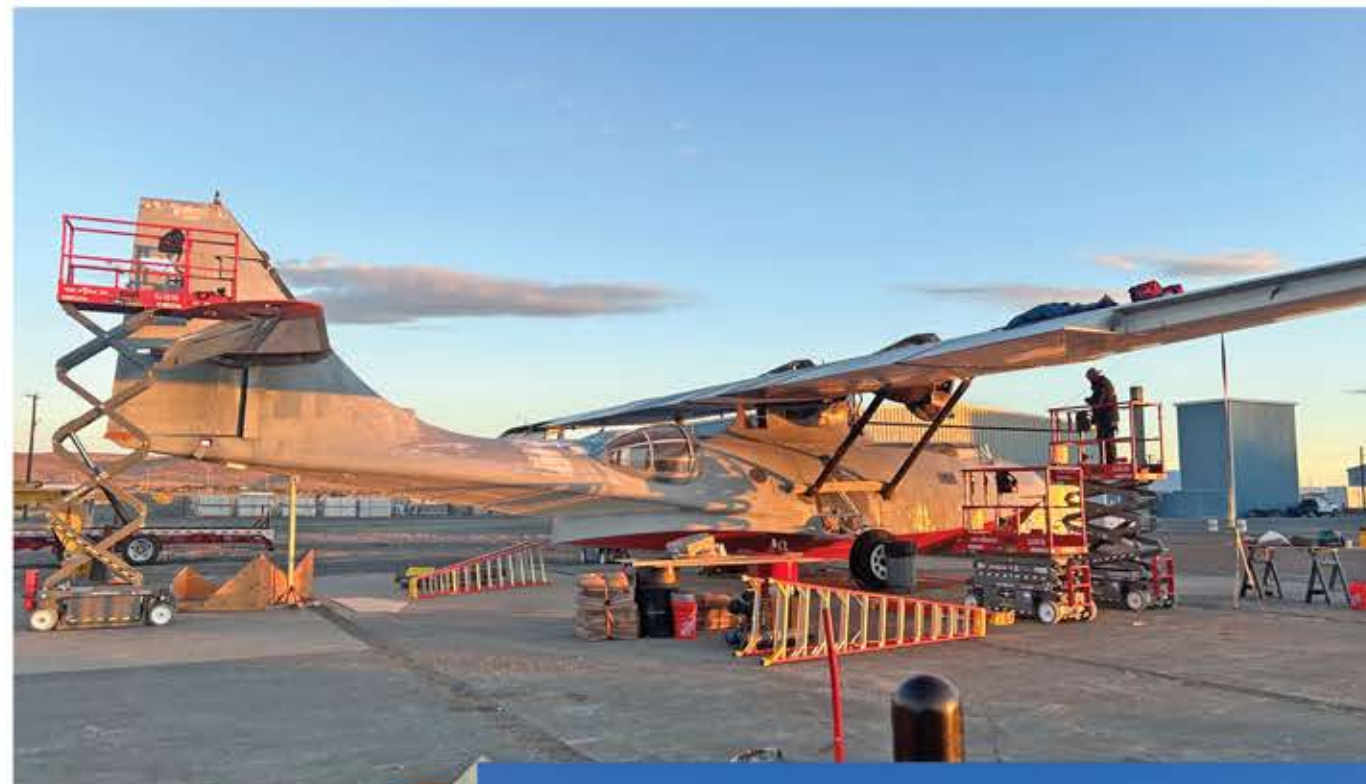
Wright R-2600 engines off, work begins on removing the wing from the pylon — no easy task. (Milo DeGrassi)
