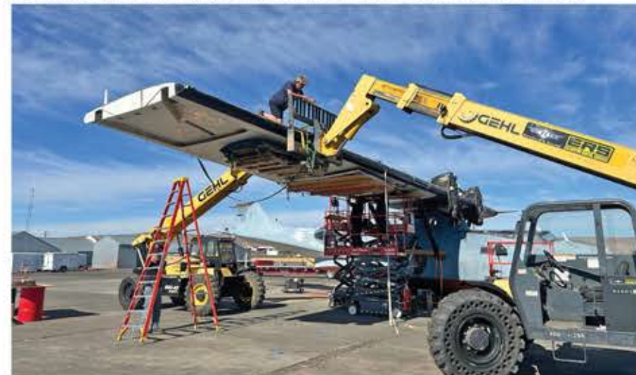
Easy does it — with the retractable floats and leading edges removed, the difficult task of lifting the wing off the pylon is underway. (Milo DeGrassi)
