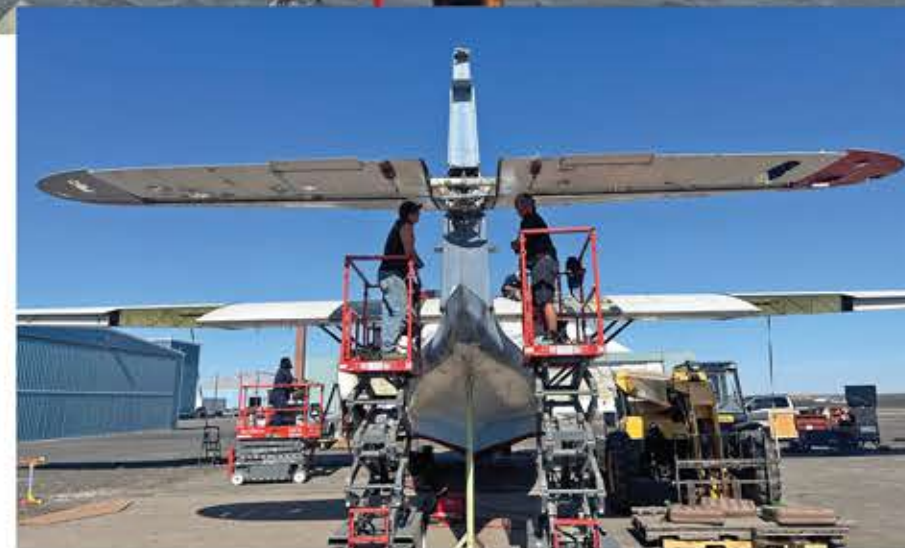
Removing the elevator and the Steward-Davis Super Cat rudder. (Milo DeGrassi)
