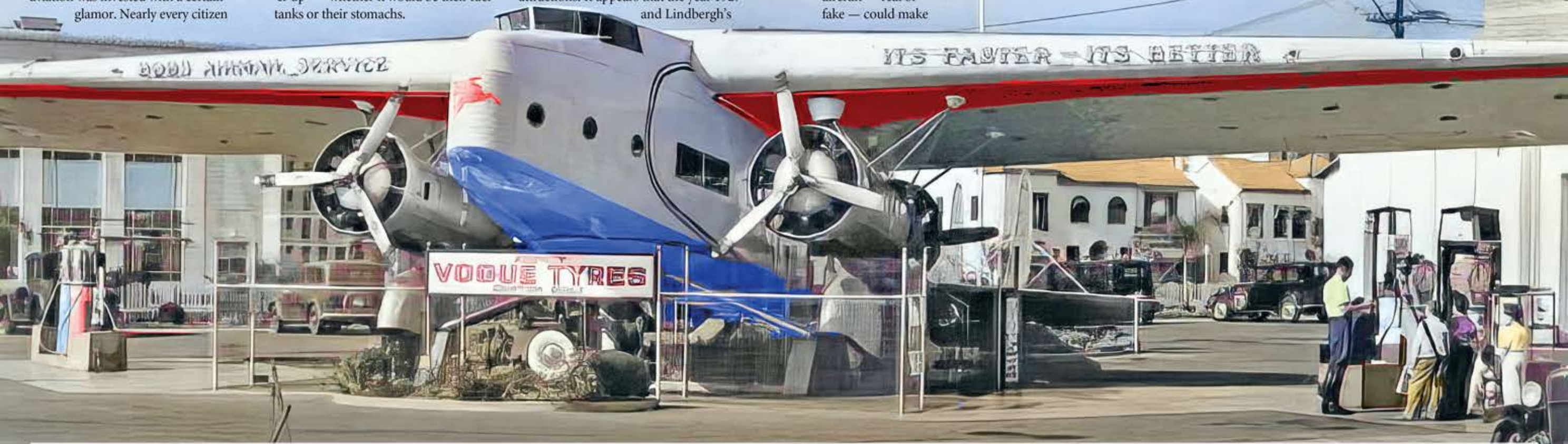
One of the most ambitious uses of an aircraft as a roadside business attraction was this Fokker F-32 airliner. For Fokker, the F-32 was a real flop. Built with fuselage of steel tubing with wood formers and fabric covering, the 99-ft wing was all-wood and that was a real point of weakness with all Fokker airliners of the period. The designation F-32 came about because the plane was designed to carry 32 passengers, which was a really big load for the time. Basically, all such aircraft were underpowered and the way Fokker figured out to get around this was to install back-to-back engines with one pulling and one pushing.
