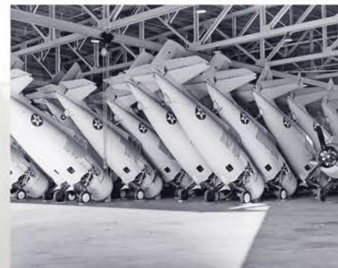
The Grumman Wildcat was in full production when the Japanese attacked Pearl Harbor. These USMC Wildcat fuselages were photographed at the factory prior to mating with their wings.
