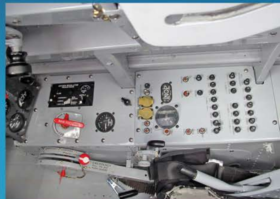
Right side console in Furias with the emergency landing gear control at the bottom. (MW)
