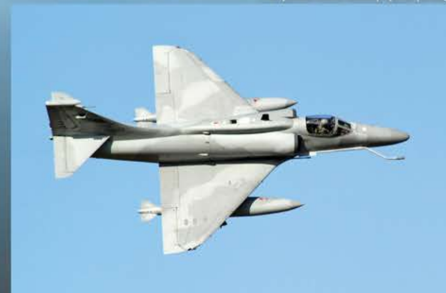
Fightinghawk in a pass that displays the additional aeriels and refueling boom.
