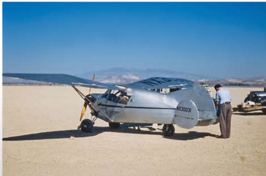
Surviving specifications indicate the Plane-Mobile had a fuselage/car length of some 16 feet while the wing, when fully spread, spanned 35 feet. When the wing was folded, the contraption would sort of scuttle down the road and, as one spectator put it, the Plane-Mobile "had all the grace of a hermit crab."
