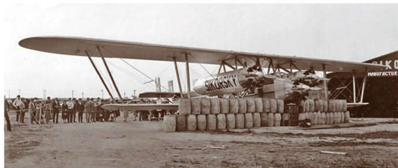
The Sikorsky S-35 photographed with the amount of fuel and oil needed for the transatlantic flight (some 15,200-lbs). With wing and fuselage tanks full, nearly half this load was stored in the cabin, which measured some 15 feet in length.
