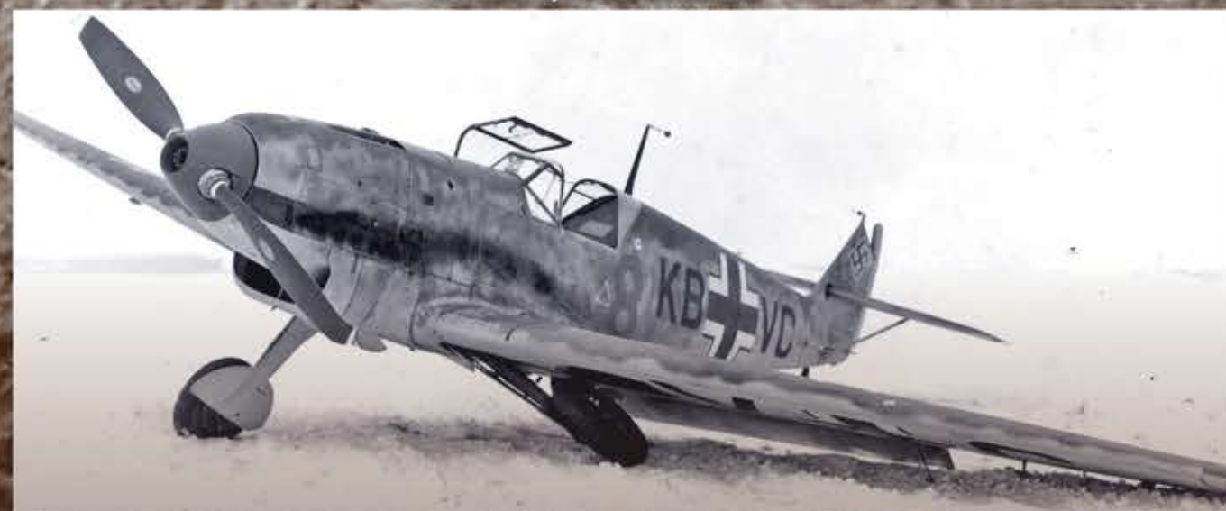
An early Bf 109D-1 carrying the fuselage codes KB+VC fell victim to a ground loop on a snow-covered airfield in Germany. The two-blade propeller is shown to advantage.
